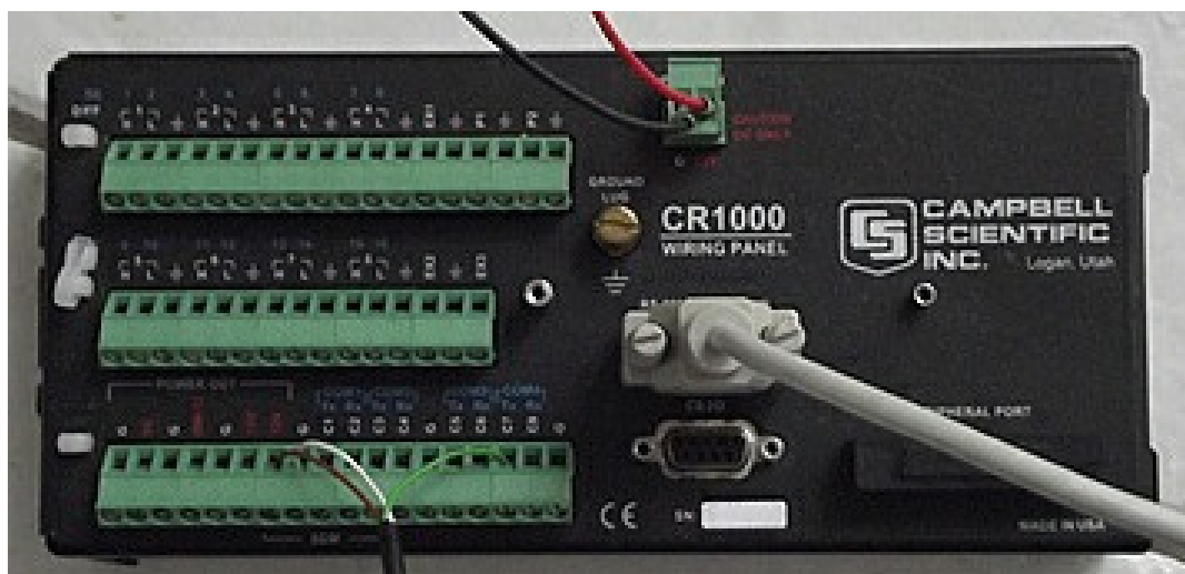
Figure 1: Campbell Scientific datalogger CR1000
